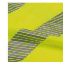
segmented retroreflective bands
